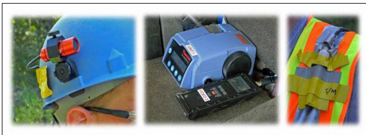
Figure 1. (from left to right) Video camera attached to helmet, dust monitor and video monitor, and safety vest to hold instrumentation.
