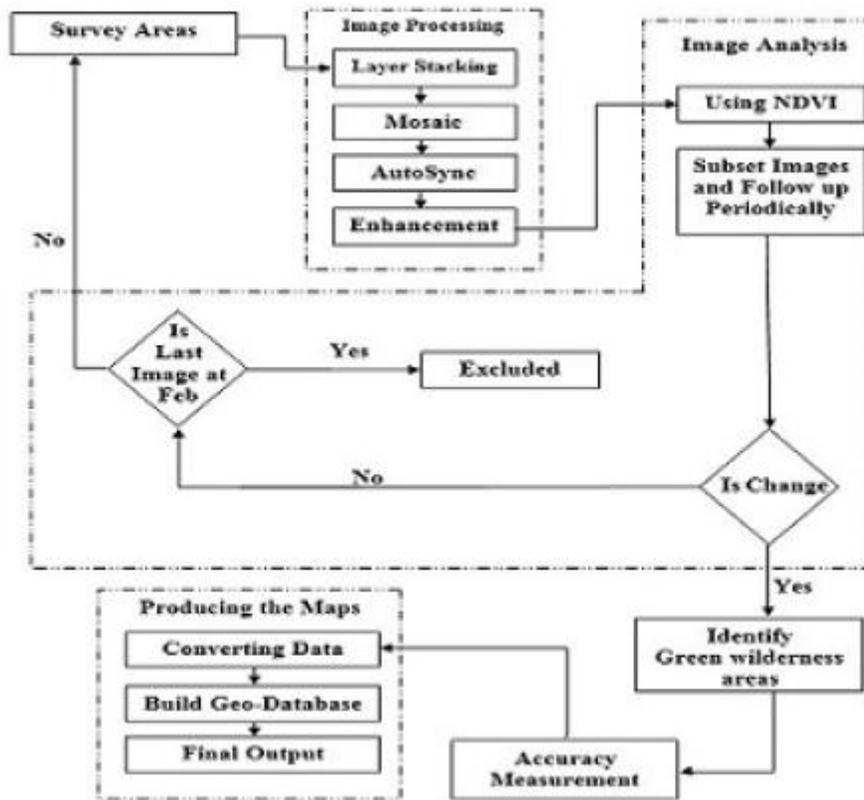
Figure 1: Image Detection Algorithm
