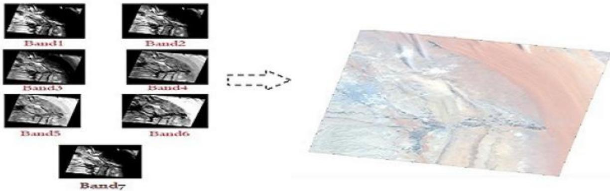
Figure 4: Layer Stacking Proces
