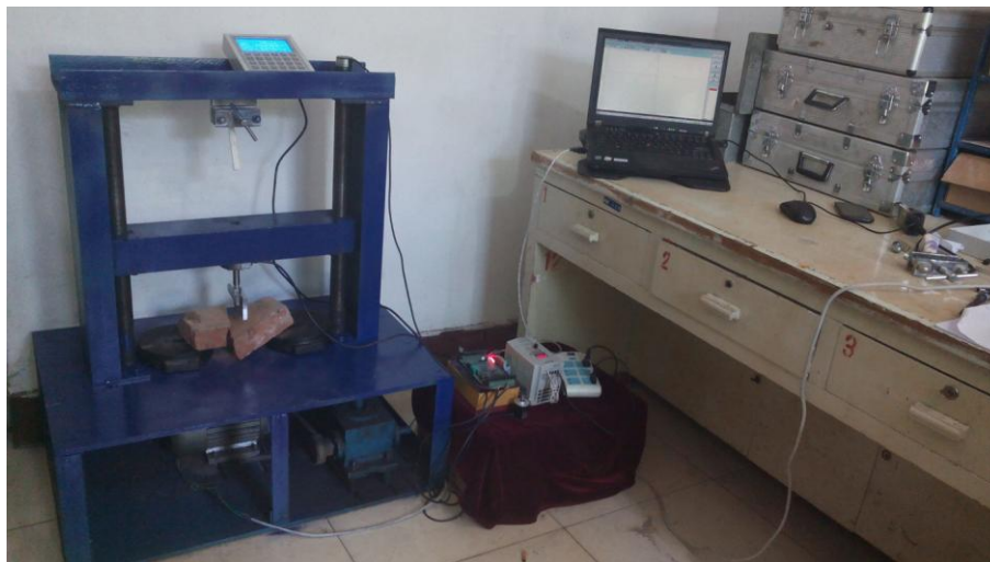
Fig 2: The experimental set-up photograph of brick measurement.
