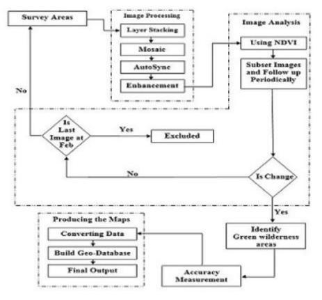
Figure 1: Image Detection Algorithm
