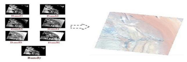
Figure 4: Layer Stacking Proces
