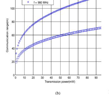
Fig.1: Enhancement of communication range for (a) path loss exponent  $\gamma = 3.0$  (b) path loss exponent  $\gamma = 3.5$
