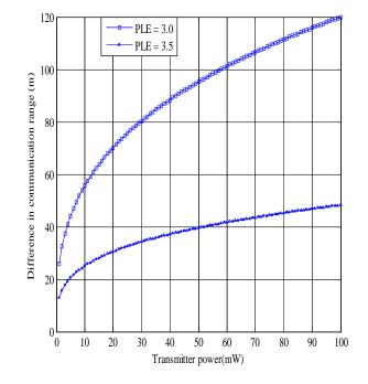
Fig. 2: Difference in communication range for conventional and CR enabled sensor nodes
