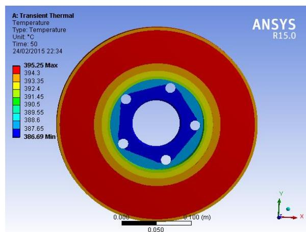
**Fig.3: Results of thermal analysis of perforated model Fig.4: Results of thermal analysis of simple model**
