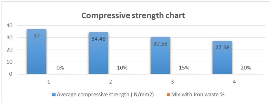
**Fig 8: Compressive strength test results on concrete**
