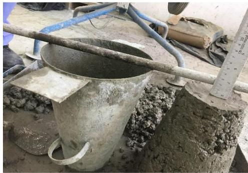
Fig 5: Slump Test
