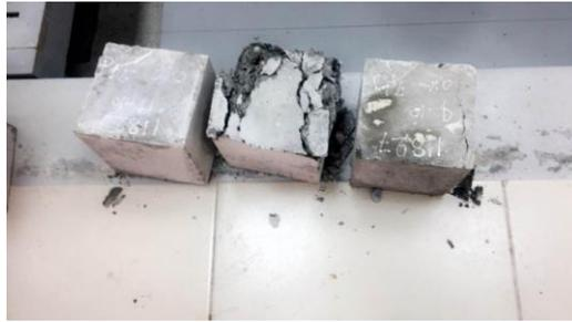
**Fig 7: Compressive strength test on concrete**
