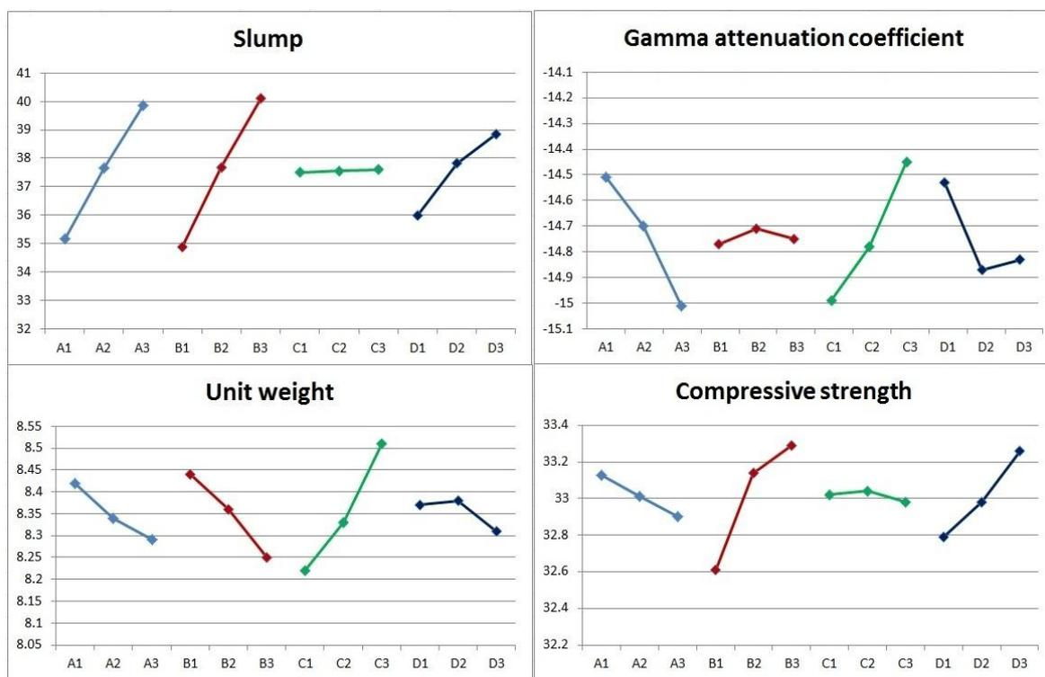
Fig. 3- The S/N ratios of each level for selected parameters on full responses.
