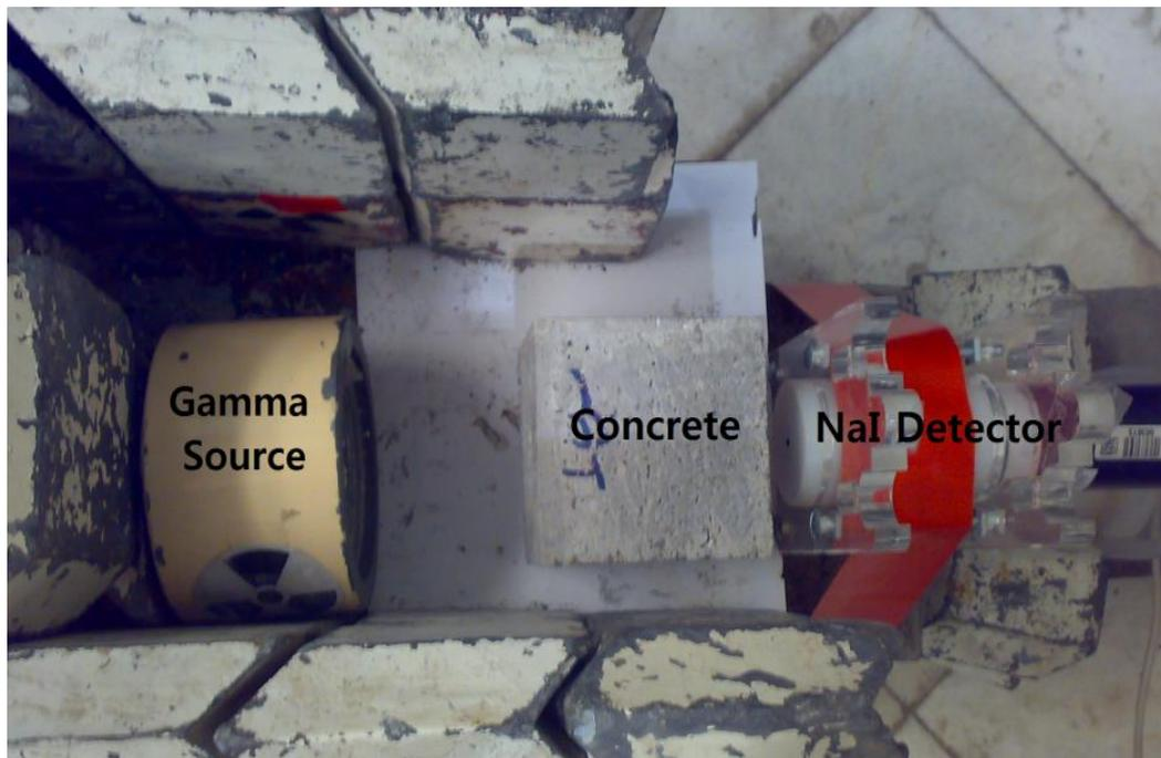
Fig. 2. Experimental setup for gamma attenuation coefficient measurement
