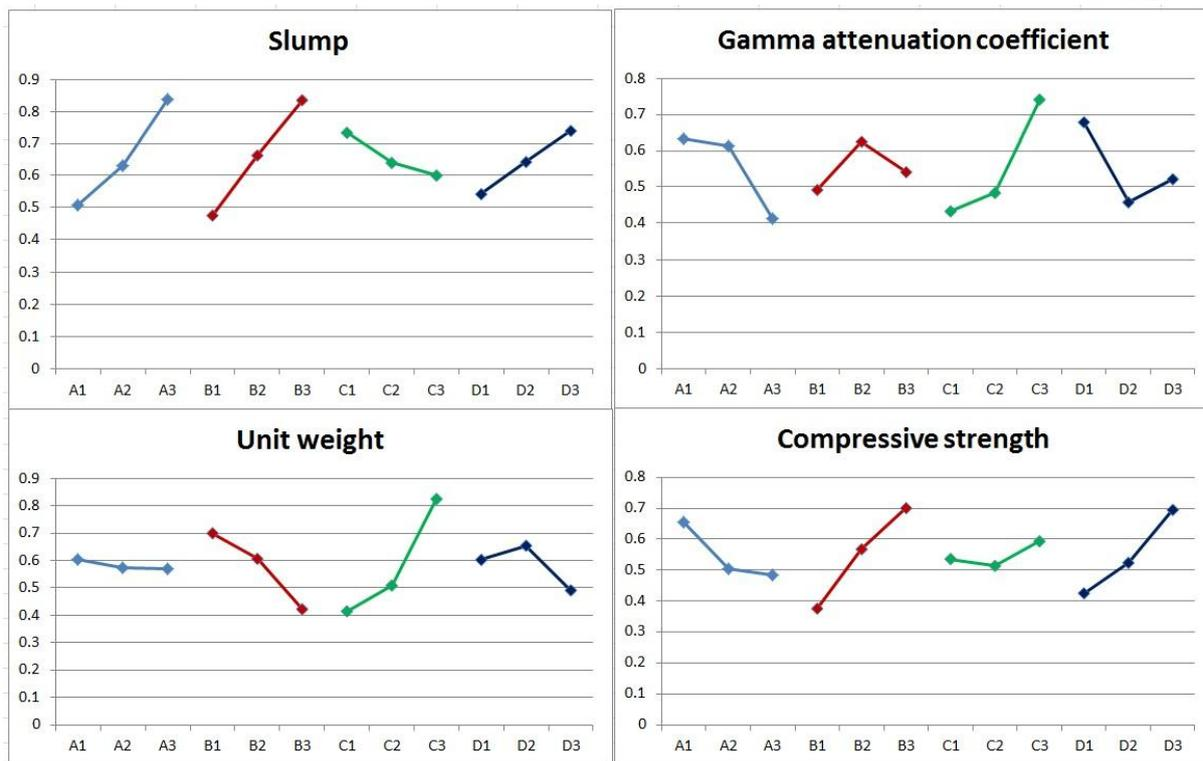
Fig. 4- Grey relational coefficients of each level for selected parameters on full responses.
