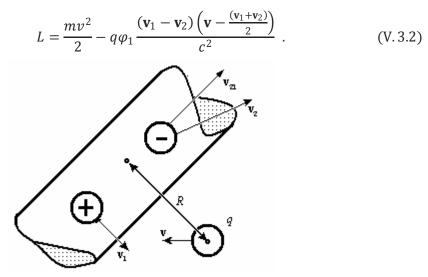
Fig. 6Notation:  $\mathbf{v}_1$  is speed of positive charges of a conductor (ions);  $\mathbf{v}_2$  is the velocity of conduction electrons of the conductor; v is the free charge,  $\mathbf{v}_{21} = \mathbf{v}_2 - \mathbf{v}_1$  is the average velocity of the conduction electrons in the conductor.
