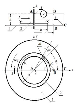
Fig. 9. 1 is conducting disk; 2 is a ring with a current; 3 is sliding contact.
